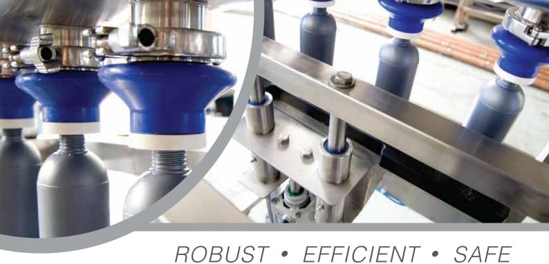
*Filtec Automation* offer a Semi Automatic level filler to fill free flowing low viscosity products; such as milk, water, beverages, cordials, vinegars etc. Included is a tank that will hold approximately 60 litres. The level filler is also offered with an option of a level control which will be fitted to the inside of the tank.
